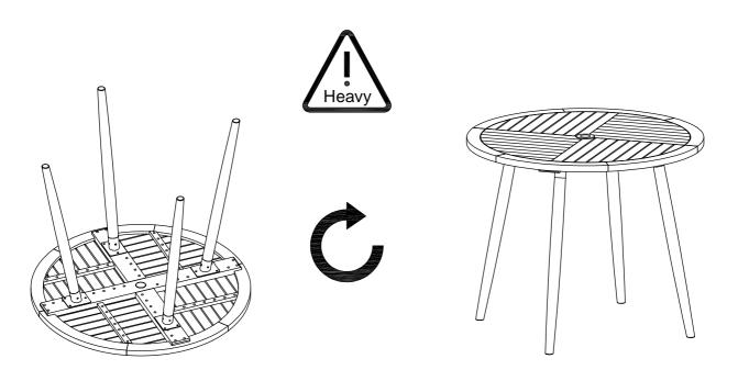
With 2 people, carefully turn and place the table on its feet. Take care when lifting not to damage the legs.
