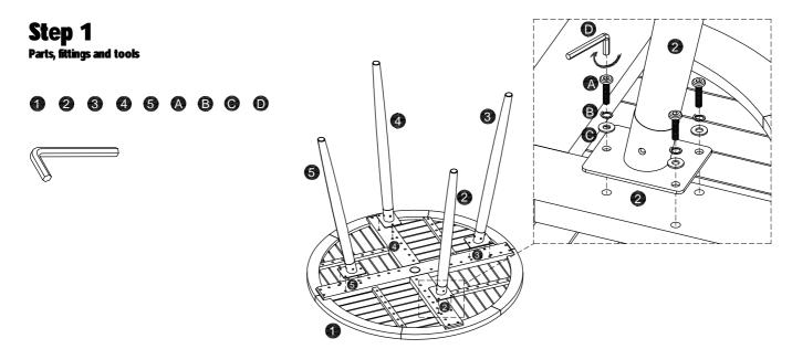
Find a clear area for assembly, near where you intend to use the table. Place table top (1) upside down on a soft surface. Then take the leg (2),(3),(4),(5), turn it upside down and align it to the hole position (2), (3), (4), (5) on the table top (1). For each hole, combine together x 1 Allen bolt (A), x1 Lock washer (B) and x 1 washer (C) and insert into the hole, tightening with the Allen key (D) provided. Repeat this process for all legs.
