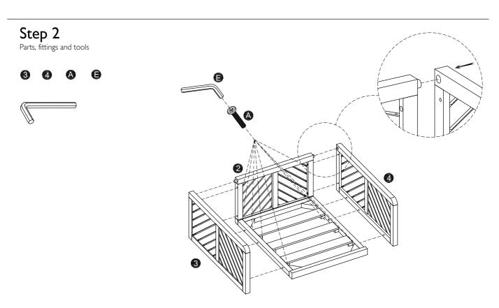
Attach the left side panel (3) and right side panel (4) by inserting the tenon located on either side of the back panel (2). For the remaining holes, insert Large allen bolt (A) and tightening with the Allen key (E) provided.
