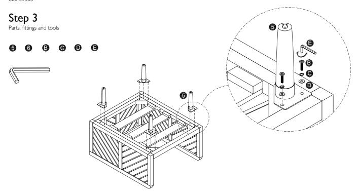
Carefully turn over the sofa to access the underside of the bottom panel. Locate the legs (5) and middle leg (6) and secure using the Small allen bolt (B), Lock washer (C), Washer (D) tightening with the Allen key (E) provided.
