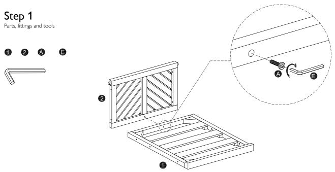
Find a clear area for assembly, near where you intended to use the armchair. Place bottom panel (1) on a soft surface and align with back panel (2). For each hole, insert Large allen bolt (A) and tightening with the Allen key (E) provided.
