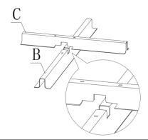
**Step 2:**Put the Upward Steel Cross Base(C) on Downward Steel Cross Base(B) and intersect at the notches.
