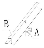
**Step 1:**Place the Cross Base Stabilizer (A) under the Downward Steel Cross Base (B) and align the mounting positions of each.
