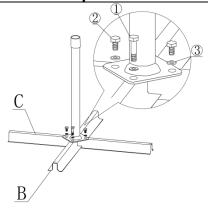
**Step 3:** Attach the Base Pole(D) and Steel Cross Base(B) using Washers(③) and Bolts(①) with Spanner.
