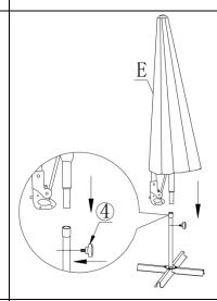
**Step 4:** Insert the pole of the Canopy Sunshade (E) into the Base Pole(D) aligning the mounting positions of (E) and (D). Screw in by hand the Screw With Acrylic Cap(4) in the mounting positions of (E) and (D) to ensure that the pole is tightly secured to the base.
