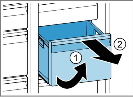
2. Lift the fruit and vegetable container cover slightly ①, pull it forwards and remove it ②.
