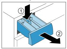
3. Pull out the insert upwards.
