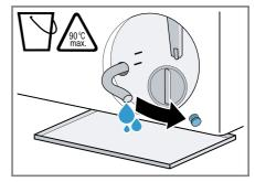
8. Firmly press on the sealing cap.
