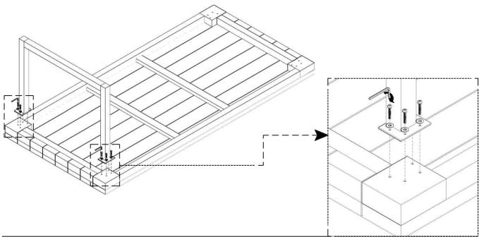
Note: Failure to tighten legs securely, will cause product to be unstable
