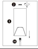
9. Remove socket rings (J) from all 3 sockets. Place 3 shades (I) onto sockets and then screw on socket rings (J) to secure shades.
