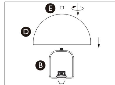
3. Place shade (D) onto harp (B) and tighten it with nut (E).
