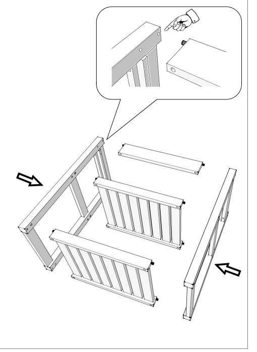
Step 4 Fix the parts together using Allen Key (H1), screws (A1) x10 and bolts (B1) x10 as shown in the diagram. Note the position of the bolts.
