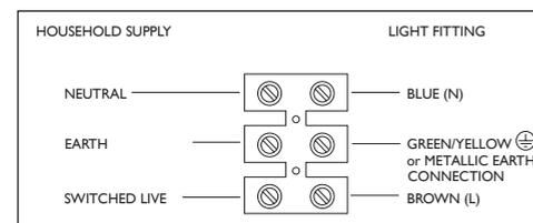
Having identified the household wiring from your existing light fitting, connect to the outdoor rated connection block (D) inside the product in the following way.
