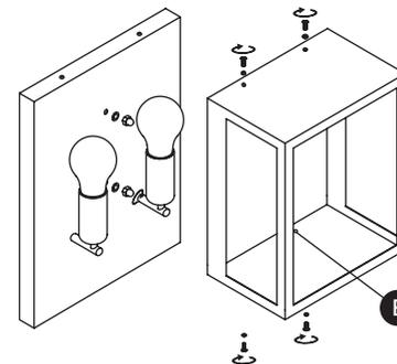
Re-attach the light fitting to the back plate (C) by locating the screw holes over the screws and replacing the rubber washers and the finials (B) and tightening them securely.
