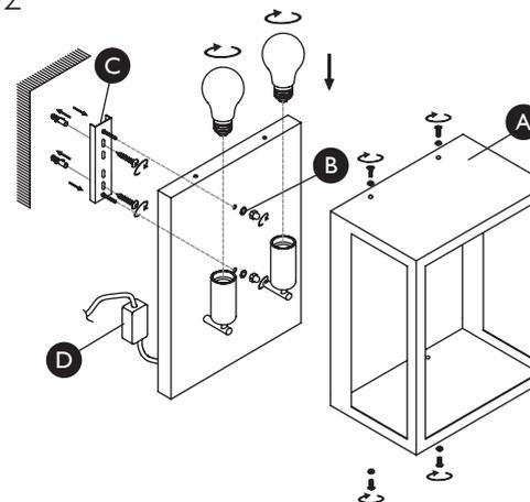
Remove the shade (A) from the product by undoing top and bottom screws and washers. Save for refitting later. Remove the back plate (C) from the fitting by removing finials and rubber washers (B).
