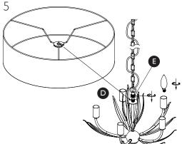
Re-attach the product to the fixing bracket and tighten the side screws.
