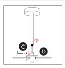
Using the Hex key provided (C) loosen the grub screw located in the receiving tube of the central hub (D) Rotate the main, threaded stem into the receiving tube (holding the receiving tube still) until hand-tight and secure in place by re-tightening the grub screw. Take care not to twist the wiring or cross-thread the tube.
