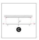
Excess cable must be carefully located inside the ceiling cup or within the ceiling cavity itself. Carefully offer fitting (C) over mounting bracket then secure in place with the screws and any washers removed earlier. Take care not to damage the wiring.
