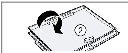
3. Press the fastenings for the lower glass plate outwards.
