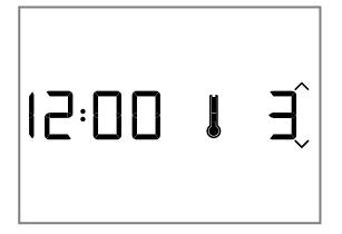
After starting operation, the thermometer on the right next to the time display shows the heating up progress of the interior temperature. The thermometer gradually lights up as the appliance heats up. When the thermometer is fully lit, the appliance has reached the set temperature. When using the grill, the thermometer is fully lit immediately.
