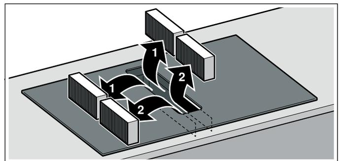
3. Insert two of the activated charcoal filters or acoustics filters into the left and right of the appliance and slide them forwards.
