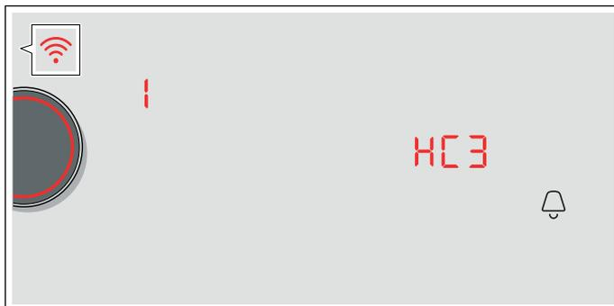
4. Set the value to **0** using the twist knob. This deactivates Wi-Fi; the
