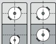
The front and rear hotplates each have two inductors and can be used independently of each other. Select the required heat setting for each of the hotplates. Use only one item of cookware on each hotplate.
