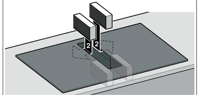
4. Insert the other activated charcoal filters or acoustics filters into the left and right of the appliance.
