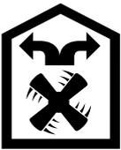
The air which is drawn in is cleaned by the grease filters and an activated carbon filter and conveyed back into the kitchen.
