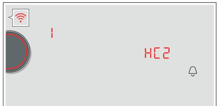
6. Start the app on the mobile device and follow the instructions for automatic network registration. The registration procedure has been completed once the
