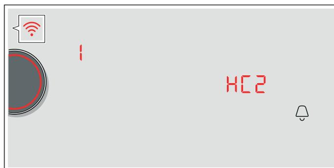
6. Start the app on the mobile device and follow the instructions for manual network registration. The registration procedure has been completed once the
