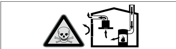
Non-room-sealed heating appliances (e.g. gas-, oil-, wood- or coal-burning heaters, continuous flow heaters or water heaters) draw in combustion air from the room in which they are installed and discharge the exhaust gases outdoors through an exhaust gas system (e.g. a chimney).
