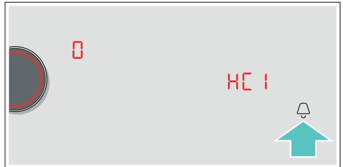
4. Use the twist knob to set the value to **!**. In the control panel, **!** and the symbol
