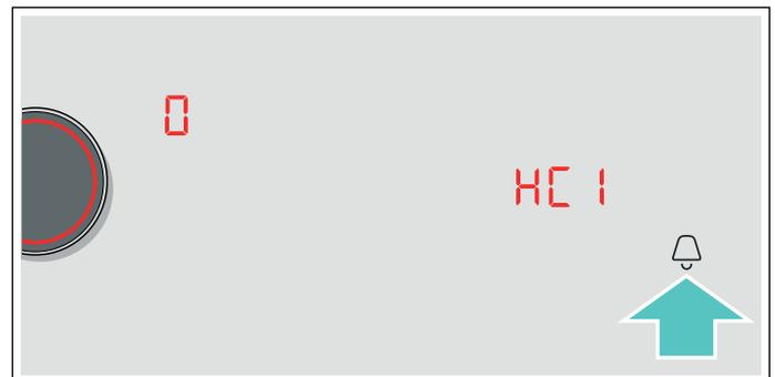
4. Using the twist knob, set the "Connect automatically" **1** value or the "Connect manually" **2** value.
