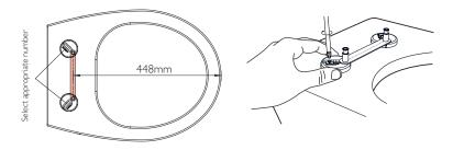
Once secured in place, remeasure the 448mm to check and remove the template. Attach the cover cap over each anchor and then click the seat in place.
