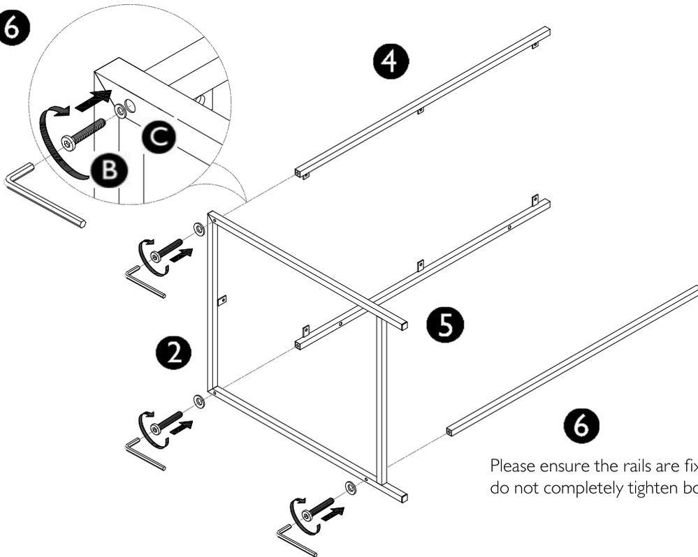
Please ensure the rails are fixed as shown, and do not completely tighten bolts at this stage.
