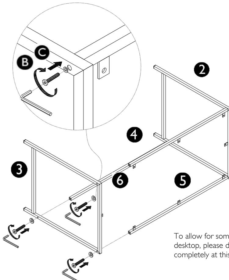
To allow for some tolerance for fixing the desktop, please do not tighten bolts completely at this stage.
