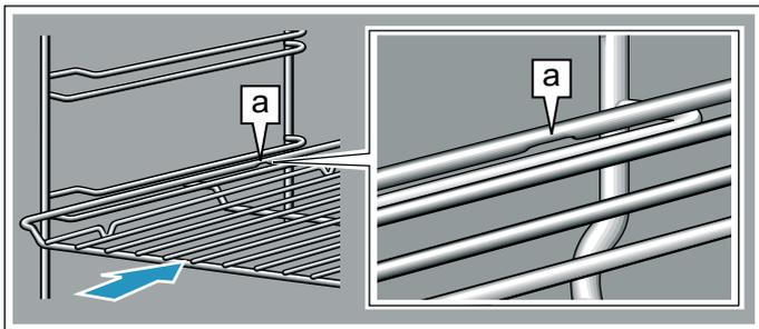
When inserting baking trays, make sure that the recess **a** is at the rear and is facing downwards. The sloping edge of the accessory **b** must be facing towards the appliance door.
