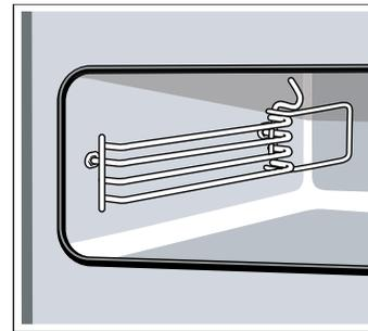
1. Lift the shelf support slightly at the front **a** and detach it **b** (fig. **1**).
