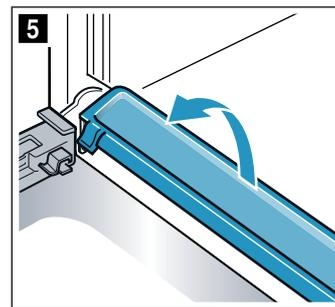
Clean the panels with glass cleaner and a soft cloth. Wipe the condensate trough with a cloth and some hot soapy water.
