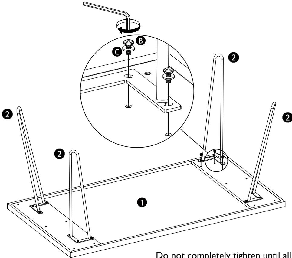
Do not completely tighten until all bolts are inserted and the legs are in the correct angle.
