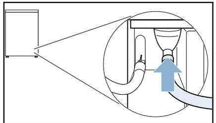
6. Secure the other side of the drain hose using the remaining accessories, depending on the connection situation.
