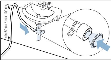
The connection point must be secured using a hose clamp (12-22 mm clamping range, available from specialist retailers). When connecting to a siphon, make sure that the drain hose is routed at a height of at least 80 cm, but no more than 100 cm.
