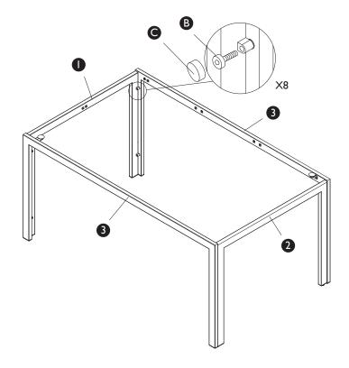
**IMPORTANT:** Tighten the screws with hand only. Do not fully tighten until the end of step 2.
