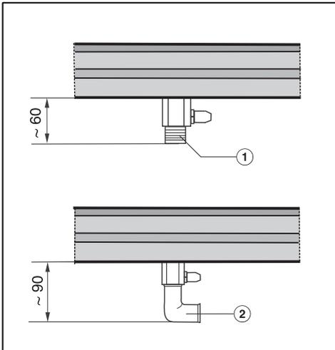
① Connection R  $\frac{1}{2}$ " with test point - ISO 7-1 (DIN EN 10226)
