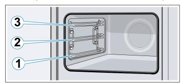
When using positions 1, 2 and 3, always insert the accessory between the two guide rods for a shelf position.
