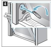
Left lock: Anti-clockwise Right lock: Clockwise
