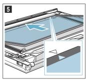
Push the intermediate glass panel downwards in area b, insert holder c at an angle and push down until it locks into place (Fig. 6).
