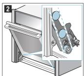
3. Turn the door handle upwards slightly **a** so that the appliance door slides downwards fully **b** (Fig. 3).
