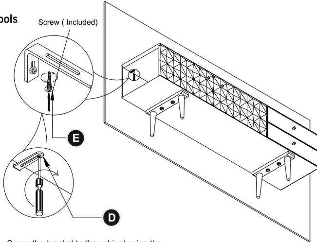
Screw the bracket to the cabinet using the pre-drilled hole with screw provided
