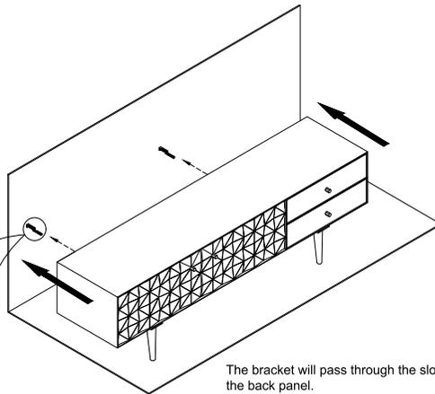
The bracket will pass through the slots in the back panel.
