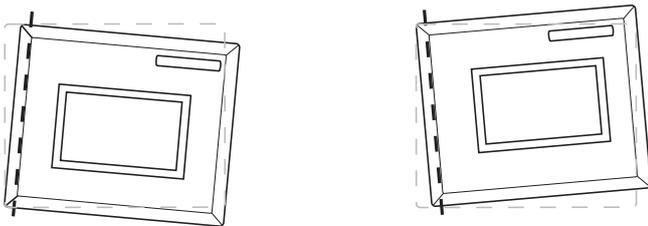
Effect of hinge adjustment – exaggerated for clarity
