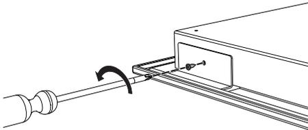
6. **Only for models with lateral UR:** pull out the bracket.
