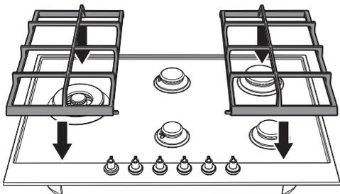
2. Lay the centre grid engaging the notches in the teeth of the lateral grids.
