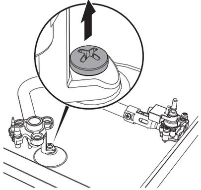
2. Remove the burner work surface and the corresponding gas supply hose.
