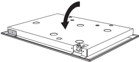
5. **Only for models with lateral UR:** remove the bracket fixing screw.
