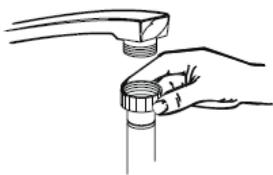
Connect the cold water supply hose to a threaded 3/4(inch) connector and make sure that it is fastened tightly in place. If the water pipes are new or have not been used for an extended period of time, let the water run to make sure that the water is clear. This precaution is needed to avoid the risk of the water inlet to be blocked and damage the appliance.
