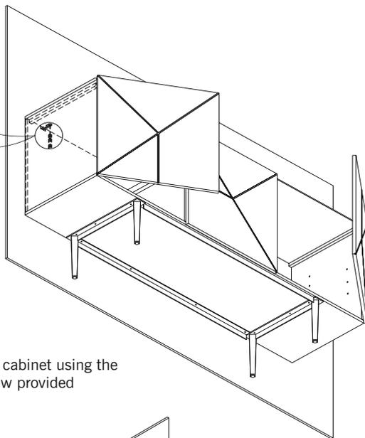
Screw the bracket to the cabinet using the pre-drilled hole with screw provided
