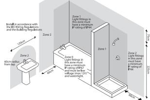
This product has special protection against the ingress of moisture and is IP44 rated. This product is suitable for use in Zone I. Zone 2. and outside Zones of a bathroom. See diagram. If installing in a bathroom a 30mA RCD must be used in accordance with IEE Wiring Regulations and the Building Regulations.
