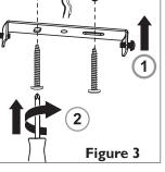
Attach to the ceiling using the screws provided. Refer to Fig. 3. Ensure there is a joist at the point of fixing to support the weight of the product. Take care to avoid damaging any concealed wiring and pipes.
