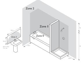
This product has special protection against the ingress of moisture and is IP44 rated. This product is suitable for use in Zone I, Zone 2, and outside Zones of a bathroom. See diagram. If installing in a bathroom a 30mA RCD must be used in accordance with IEE Wiring Regulations and the Building **Regulations.**
