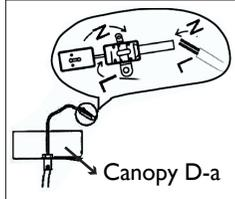
Having identified the household wiring from your existing light fitting, connect to the connection block inside.
