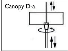
If necessary, loosen the small piece D-c and move the cable D-b to adjust the height of the pendant lamp. Then tighten the piece D-c again.
