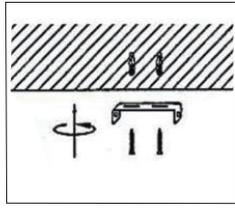
Fix the metal bracket to the ceiling, ensuring there is a joist at the point of fixing to support the weight of the product.
