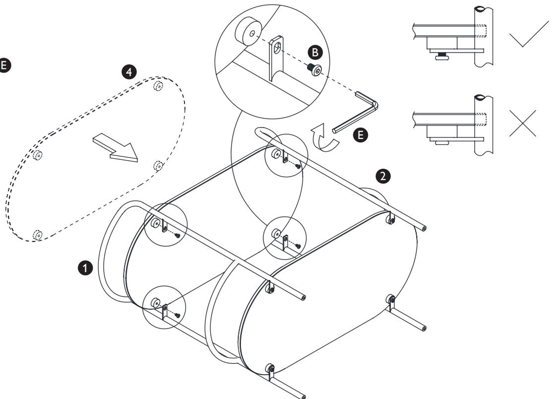
With 2 people carefully support the glass (4) and align with the brackets located on the frame. Insert the allen bolts (B) with the allen key (E). Do not fully tighten at this stage until the trolley has been placed on its wheels to ensure the item is level.
