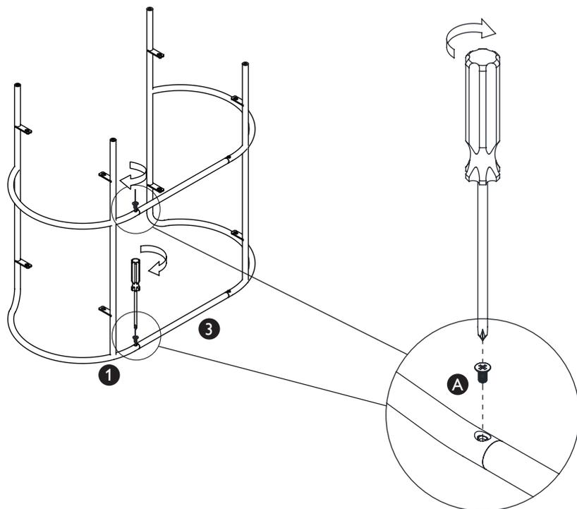
Fix the connecting bars (3) to the leg (1) using the screw (A) and the screwdriver.
