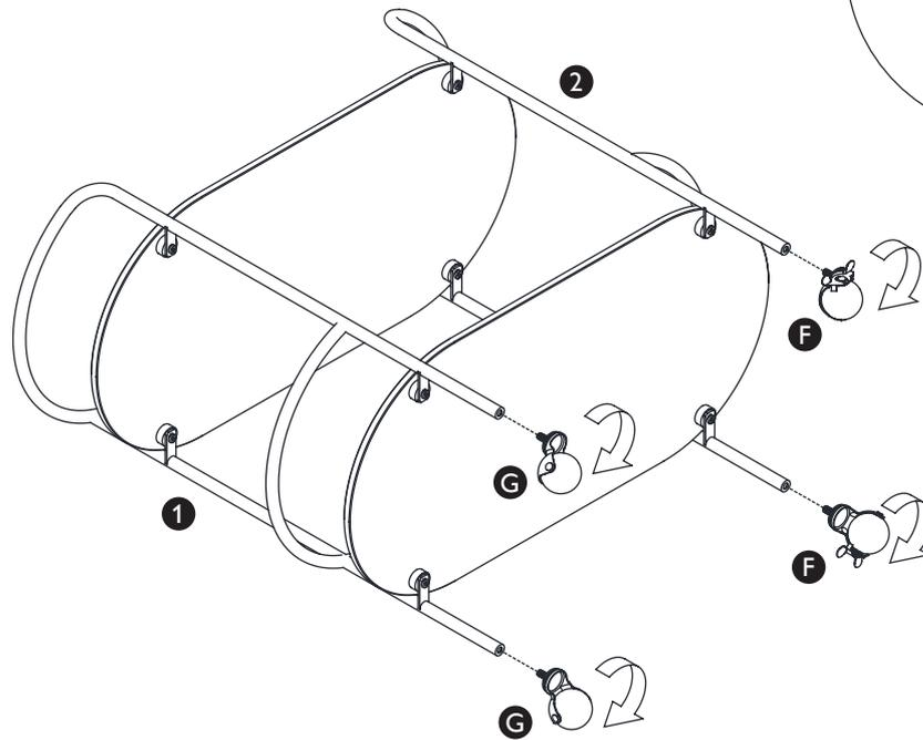
To fit the wheel, rotate this collar clockwise
