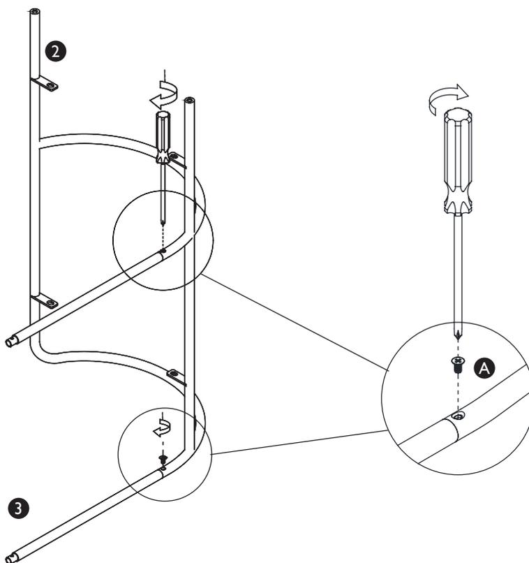
Fix the connecting bars (3) to the leg (2) using the screw (A) and the screwdriver.
