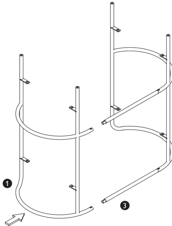
Locate the leg (1) onto the connecting bars (3) as shown above.
