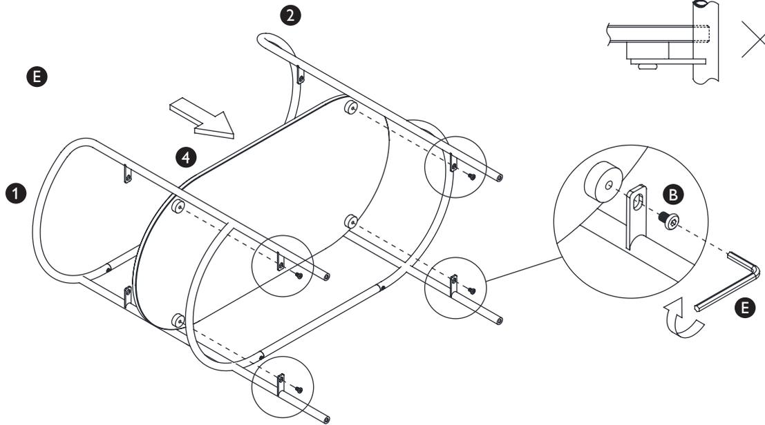
With 2 people carefully lay the trolley on its back on a soft surface. Support the glass (4) and align with the brackets located on the frame. Insert the allen bolts (B) with the allen key (E). Do not fully tighten at this stage until the trolley has been placed on its wheels to ensure the item is level.
