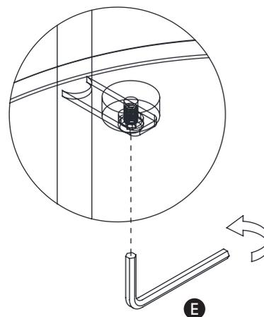
With 2 people carefully place the trolley onto its wheels. With the allen key (E) firmly tighten all the allen bolts.
