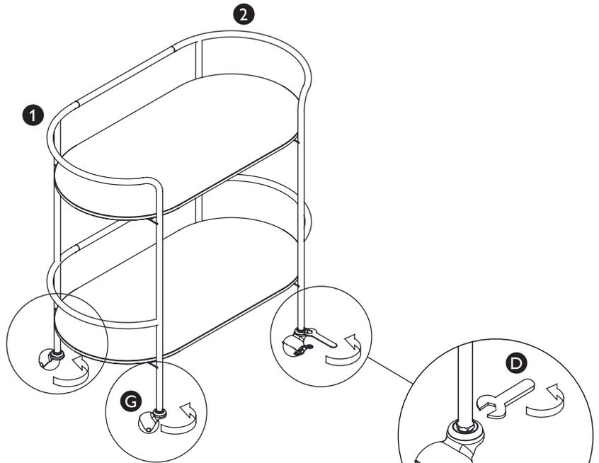
Using the open end spanner (D) firmly tighten the wheel nuts as shown in the detail above. Should the trolley require a small amount of levelling remove the necessary wheel and install a washer (C). Refit the wheel and tighten securely.
