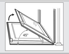
Step 4 Hold the door trim (B) on the top edge of the door at the two sides and push inwards to release the clip seal.
