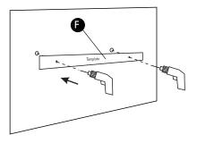
Step 1 Place template (F) on the wall. Please use a spirit level to ensure that the template is straight. Drill the required holes in the wall using the template and follow the guidance on the 'Wall Fixings' section.
