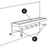
Step 9 Screw in the two additional hooks (B) by hand.
