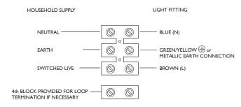
**Check that.....**You have correctly identified the house wires. The connections are tight.
