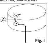
chain links. The slack electrical cable can be reduced and secured by pulling the cable through the cord grip (A). Always ensure that the weight of the product is supported by the chain and not the electrical cable.
