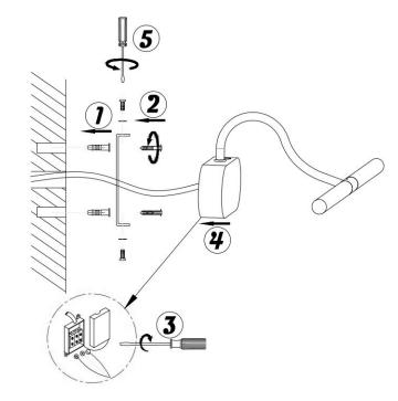
Ensure electrical connections are tight and no loose strands of wire are left out of the connector block.
