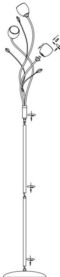
**Step 1:** Screw the centre pole section and the lamp head section of the fitting together taking care to hold the parts parallel so that they do not cross thread. If in doubt, undo and start again. Keep the lampholder section still and only rotate the lower pole to prevent twisting of the cable.
