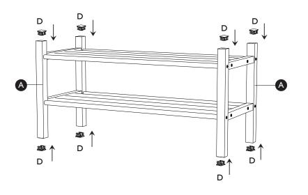
4. Insert 8  $\times$  plastic cap (D) on the top and bottom of 2  $\times$  side frame (A).
