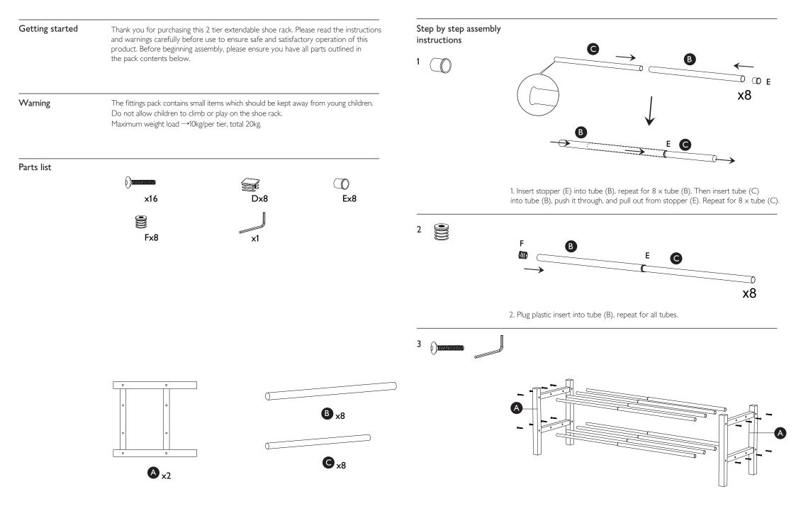
3. Affix the tube (B+C) to 1 × side frame (A) using 8 × screw . Repeat for the other side frame (A).
