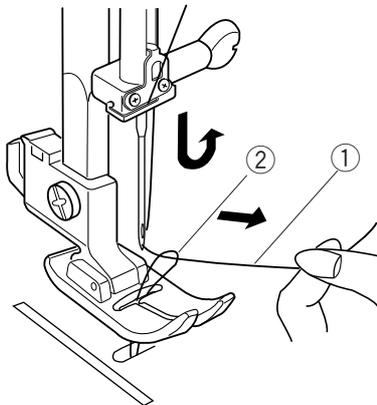
2 Turn the handwheel slowly toward you one complete turn. Bring the bobbin thread up by pulling the needle thread as illustrated.
