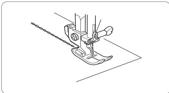
The pattern is sewn with two stitches forward and one stitch backward, forming a seam that does not rip easily. Use it to reinforce areas such as crotch and armhole seams.
