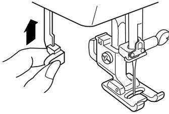
6 When buttonhole sewing is finished, push the buttonhole lever up as far as it will go.
