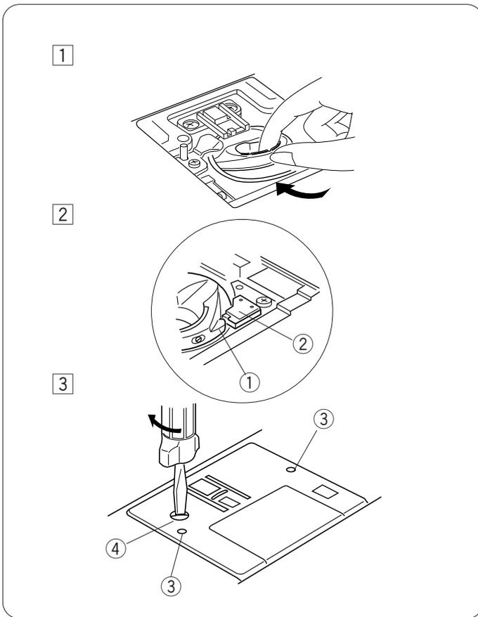
1 Insert the bobbin holder into the hook race.
