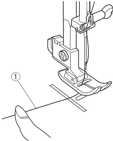
1 Raise the presser foot and hold the needle thread lightly with your left hand.
