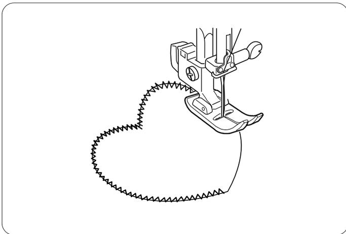
Baste appliqué pieces on the fabric, or fuse the appliqué pieces with an iron-on fabric joiner. Stitch around the appliqué, making sure the needle at the right swing falls along the outer edge of the appliqué.
