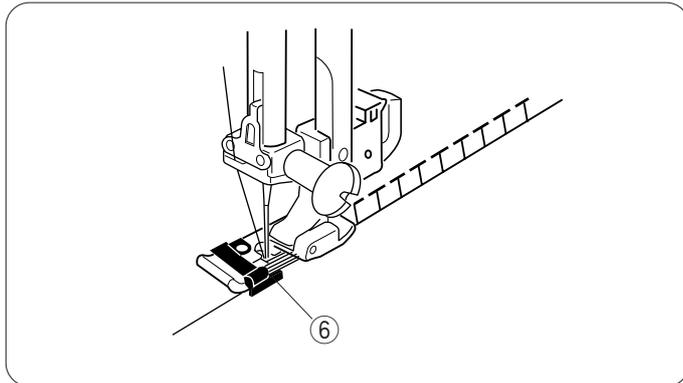
This stitch is ideal for finishing edges of stretch fabrics. It seams and finishes the fabric edges simultaneously. Place the edge of the fabric next to the guide of foot and sew while guiding the fabric edge along the guide.
