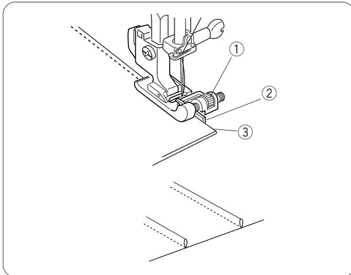
Fold a fabric wrong side together and Lower the needle into the fabric 0.1 – 0.2 cm inside the folded edge.
