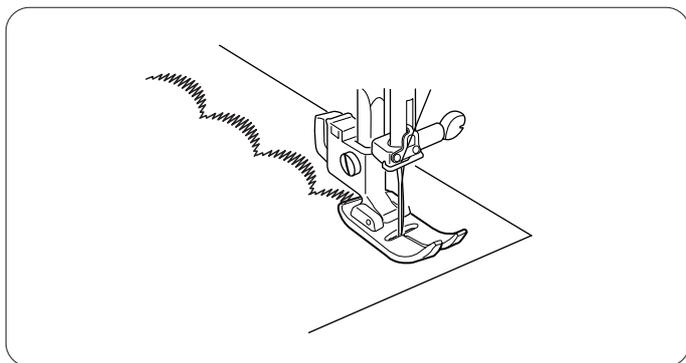
Determine the appropriate stitch density by test sewing. For a delicate appearance on fabric such as chiffon, use a single layer with a tear-away backing, if necessary. Reduce the needle thread tension slightly to achieve the better result.
