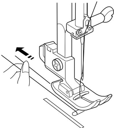
3 Pull 4" (10 cm) of both threads back and under the presser foot.
