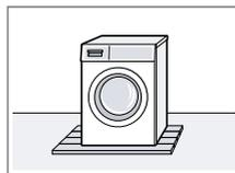
Place the appliance on a water-resistant wooden board (minimum thickness of 30 mm) which is screwed tightly to the floor.
