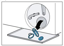
**3.** Ensure that the impeller in the drain pump can rotate.
