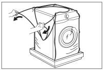
Open the door, remove the piece from the door seal and all the items from the drum.
