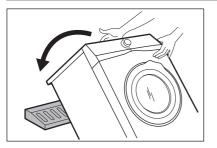
7. Remove the protection from the bottom.
