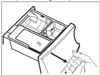
2. Put the powder detergent in the compartment . If using liquid detergent, refer to 'Filling the liquid detergent'.
