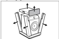
Remove the internal film.
