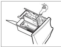
Make sure that all detergent residue is removed from the detergent conveyor. Use a cloth.
