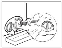
Turn the filter 180 degrees in anticlockwise direction to open it, without removing. Let the water flow out.
