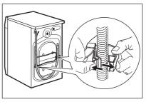
**10.** Remove the three bolts by using the spanner supplied with the appliance.
