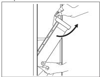
Lift and turn the drawer to pull it out of the appliance.
