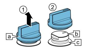
To put the control knob back on, press it on at its original position.
