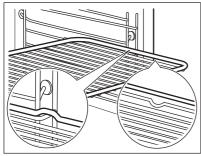
Insert the shelf between the guide bars of the shelf support. Make sure that the shelf touches the back of the oven interior.
