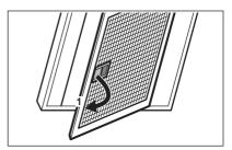
Clean the grease filters by hand using a sponge with non-abrasive detergents, or clean them in a dishwasher. We recommend cleaning the grease filters by hand.
