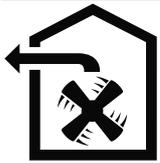
The air must not be discharged into a flue that is used for exhausting fumes from appliances burning gas or other fuels (not applicable to appliances that only discharge the air back into the room).
