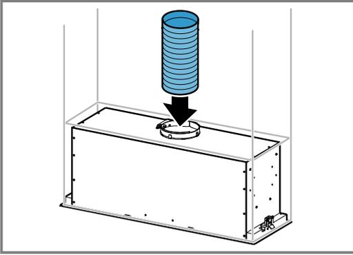
2. Establish the connection to the exhaust air opening.
